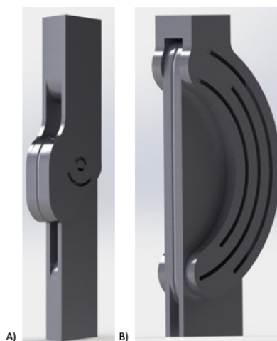
Figure 4. SolidWorks renderings of the joint design concept: A) aligned joint, B) offset joint. A tibial component with pins is shown connected to the femoral component with slots. Eyelets and cables are omitted for clarity.
