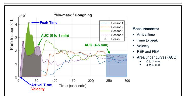
**Figure 1:** Examples of the measurements performed on the time-series data from all experiment runs for each of the four sensors and particle sizes of 0.3μm, 0.5μm, 1μm, 2.5μm, 5μm, and 10μm.
