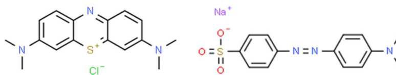
Figure 5: The MB [7-(dimethylamino) phenothiazin-3-ylidene]-dimethylazanum; chloride; and MO Sodium; 4-[[4-(dimethylamino) phenyl] diazenyl]benzenesulfonate has formula C 16 H 18 ClN 3 S and C 14 H 14 N 3 NaO 3 S, respectively.
